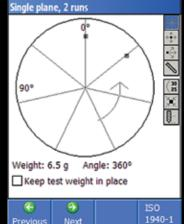
Speed measurement and High Definition Order Tracking Dynamic balancing in single plane according to ISO 1940-1
