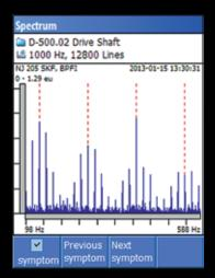
Vibration spectrum from an EVAM measurement
