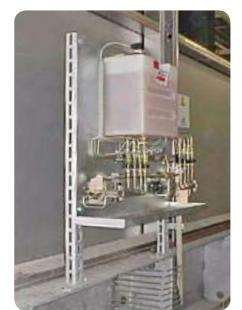
Contact-free oil lubrication with PMA2-nozzles in a paint shop
