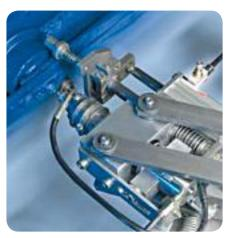
SSV and VSKH2-KR lubricant metering dividers at a conveyor belt (Beverage industry)
