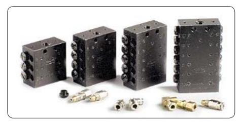
SSVD/SSVD L metering devices are adjustable per outlet pair, thus enabling a much better match to the optimum lubricant requirements. The metering occurs within the metering block by metering screws that are available in 10 different sizes.
