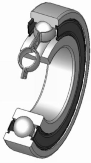
**The cages of rolling element bearings must be able maintain proper spacing of the rolling elements, have the strength to withstand centrifugal and shock forces and be able to tolerate temperature and lubricant variations.**
