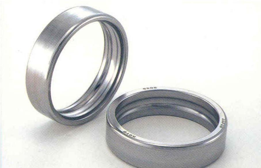
**HEAT TREATMENT** – Before the rings can be ground they need to be heat treated to provide the proper hardness, wear and fatigue resistance. At this stage the parts are either through hardened or case carburized to give the required Rockwell C level.
