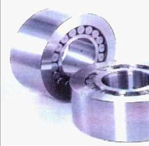
**CYLINDRICAL ROLLER BEARINGS FOR BACKING SHAFTS** – These Cylindrical Roller Bearings are designed for the backing shafts of Z-Mills and other multi-roll mills. These bearings maintain contact with the intermediate rolls supporting the roll loads. The outer rings are made of special material and are heat treated to ensure surface hardness and impact resistance for reliability.
