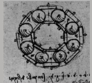
century when a horse carriage axle was fitted with a ring of balls rotating in grooves cut into the axle. With the advent of the industrial revolution during the 19th century, bearing applications were everywhere and the bearing was further developed and refined in conjunction with technology and metallurgy.
