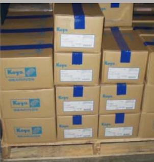
**DO** store bearings on a pallet, which is definitely a better choice than directly on the floor with no protection from moisture and vibrations from machinery.
