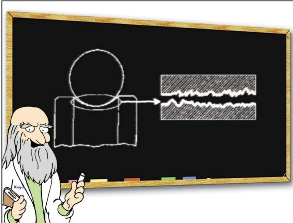
If the asperities of rolling elements and races of an anti-friction bearing come into contact with each other, a certain amount of molecular adhesion or micro-welding or shearing of these asperities as a result of the relative motion between them can be expected. The result is an undesirable surface change of the rolling surfaces. Ideal lubrication requires that an oil film be continually present to prevent contact of the surface asperities and metal to metal contact.
