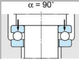
The contact angle ( $\alpha$ ) is the angle formed by the direction of the load applied to the bearing rings and rolling elements, and a plane perpendicular to the shaft center, then the bearing is loaded.
