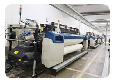
Slow rotating applications and intermittent operations are critical to the maintenance process as the quality of the fabric being woven can get affected. From handling of the most delicate construction fabrics to heavy/industrial construction fabrics, each one calls for customized attention. Contamination in semi-wet form, starches, steam ingress affects the life of bearings, lubricants and seals. Needless to say these failures adversely affect the quality and output of the fabric.
